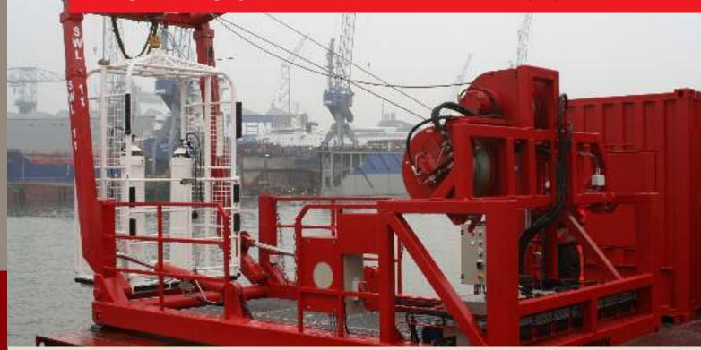
The IHC Hytech Launch and Recovery System (LARS) is a dive handling system designed to handle a dive cage with two divers with two air bottles of 50 liters. The lifting height is 100 meters.
